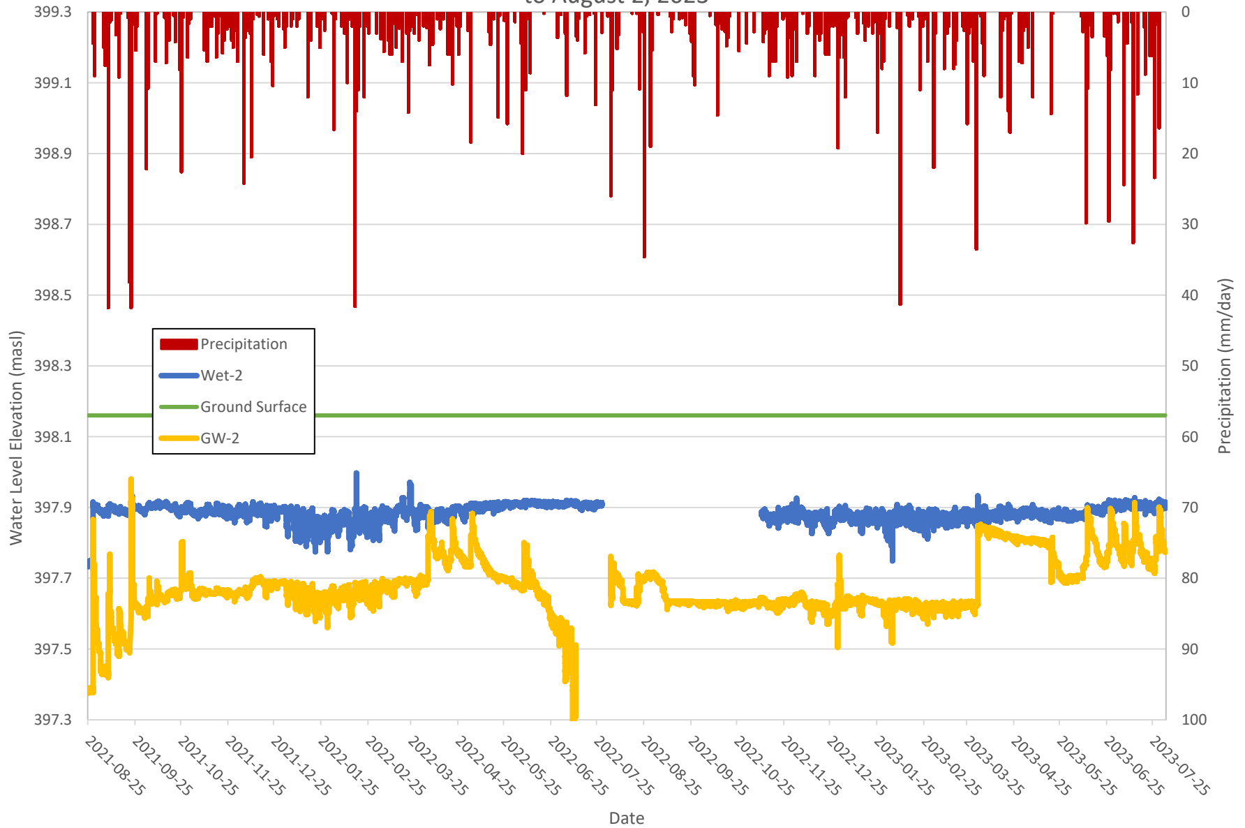
GW-2 and Wet-2 Water Level Elevation and Precipitation from August 25, 2021 to August 2, 2023
